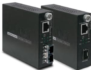
PLANET GST-80x Smart Gigabit Media Converter series extends communication distance with high Gigabit performance via fiber optic cable. The GST-80x series provides media conversion between 10/100/1000BASE-T and 1000BASE-SX/LX interfaces such as multi-mode LC/SC connectors (220m/550m), single-mode LC/SC connectors (10/20/30/40/50/70/120km) and single fiber connectors (WDM,15/60km) for various fiber optic applications.
