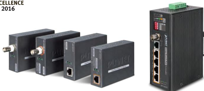
The LRP-101CE/LRP-101UE PoE Extender, which sources power from the LRP switch or LRP injector, is a Single-port, 802.3at High Power over Ethernet Injector providing a maximum of up to 25 watts of power output over Ethernet cable which allows data and power to transmit simultaneously through the cable to PoE PD (Powered Device).
