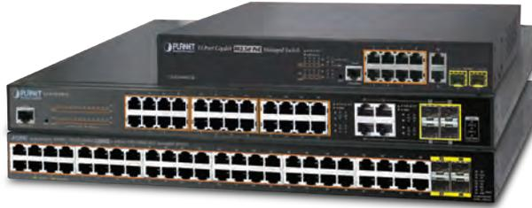
The L2/L4 802.3at/bt PoE Managed Gigabit Switches allow users to flexibly connect standard and high powered devices simultaneously. To facilitate power management, the Switches come with powerful PoE management features such as over temperature protection, usage threshold alert and auto power allocation to prevent power budget overloading. The PoE power budget can be allocated by priorities or classification and send alert event logs when power usage reaches the defined threshold.
